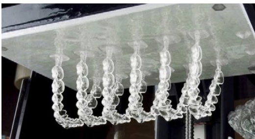
Figure 4 - Direct printed aligners in-house production
