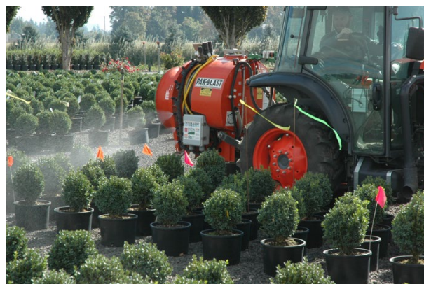
Air blast application to nursery-grown boxwood for spray coverage evaluation
