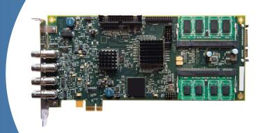
AL8xGTE-3 is a single-channel, high resolution, 8 bit 3GS/s PCI Express Digitizer board upporting the PCI Express x1 bus. Onboard memory options range from 512M samples to 2G samples Memory operation allows acquisition to continue while data is being transferred to the PC.
