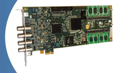
AL8xGTE-1 is a single-channel, high speed, 8 bit 1 GS/s PCI Express Digitizer board upporting the PCI Express x1 bus. Onboard memory options range from 512M samples to 4G samples Memory operation allows acquisition to continue while data is being transferred to the PC.
