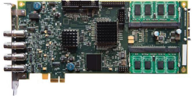
**AL8xGTE-1.5** is a single-channel, high resolution, 8 bit 1.5 GS/s PCI Express Digitizer board supporting the PCI Express x1 bus. Onboard memory options range from 512M samples to 2G samples Memory operation allows acquisition to continue while data is being transferred to the PC.
