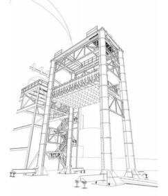
The original design concept and the real-world result of the PMLS which was utilized at a nuclear power plant located in the Midwest to lift materials and equipment 50 feet above the ground to gain access to the building's only equipment hatch.
