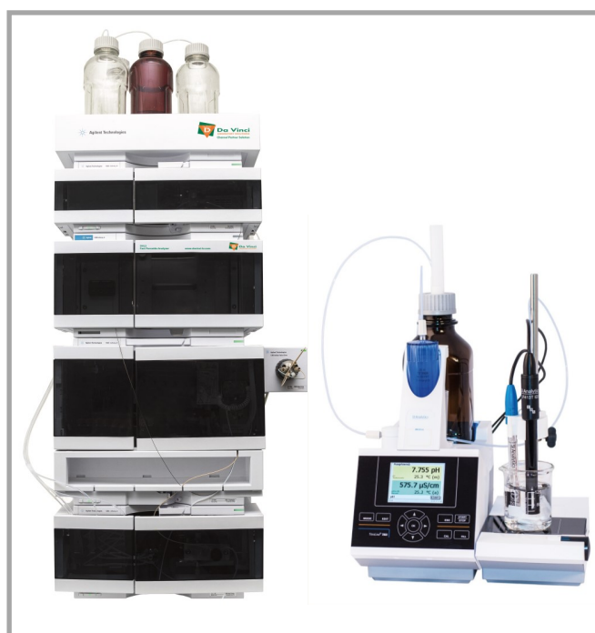
Figure One: The Fast Peroxide Analyzer versus the Iodometric Titration
