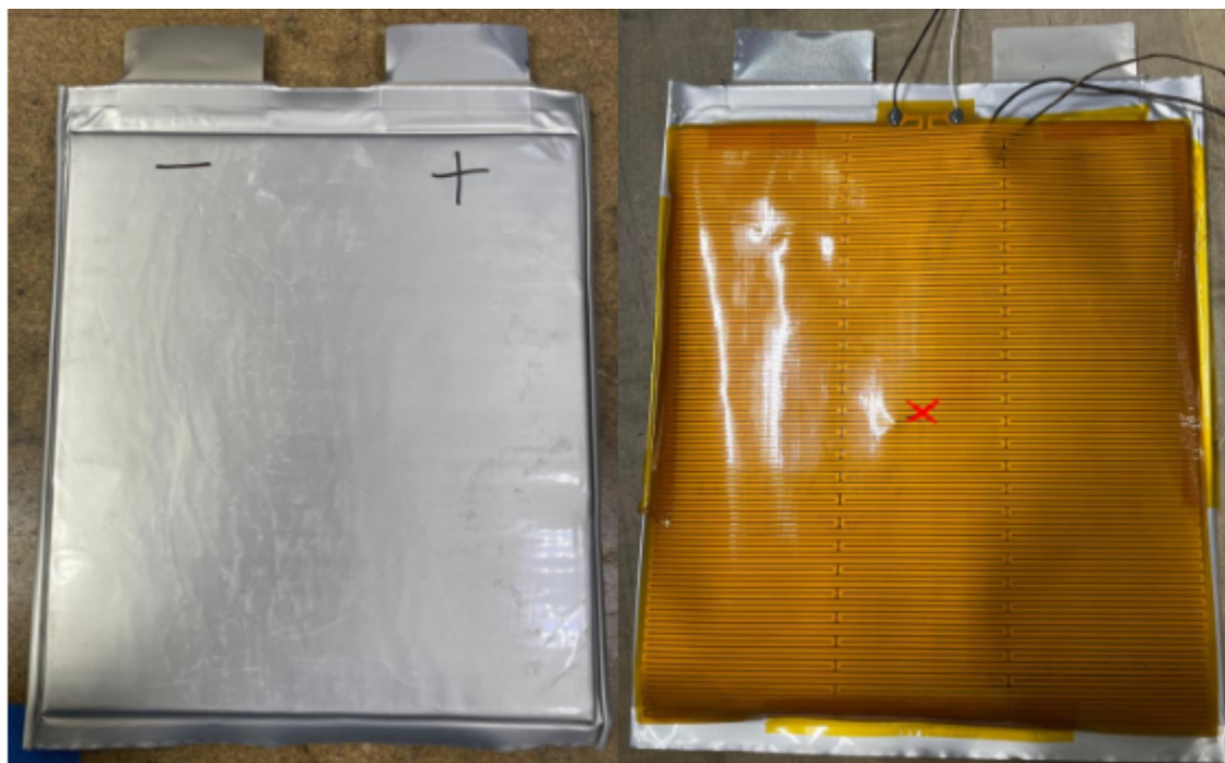
Figure 4. Individual cell tested to UL 9540A (left) and installed film strip heater (right)
