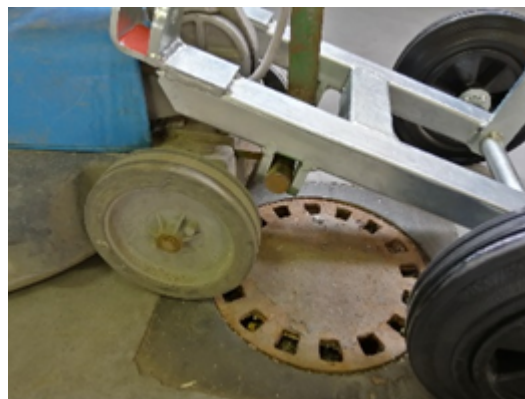
Image: Placement of the Handy Wheels with green marking downward
