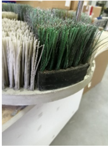
Image: Correctly mounted brush with intermediate plate
