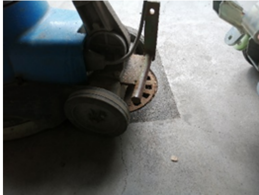
Image: The bracket at the back of the device for Handy Wheels attachment
