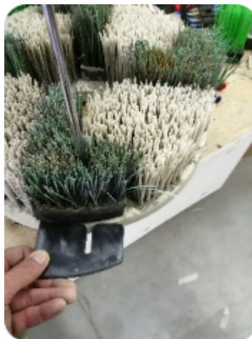
Image: Placement of the intermediate plate under the green block brush
