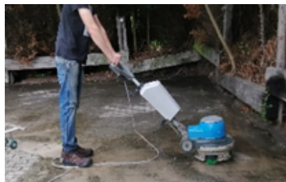
Image: Incorrect work position with the machine
