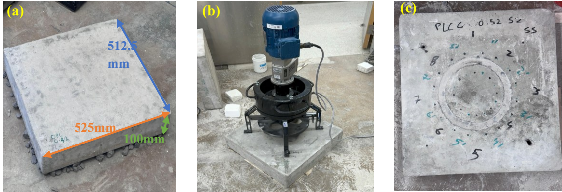
Fig. 1 —(a) Untested slab sample, (b) sample during AART, and (c) sample after AART.
