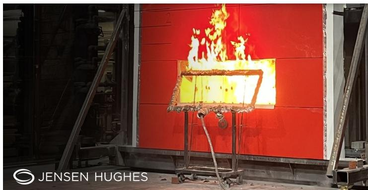
A newly completed, co-funded study has confirmed that Insulating Concrete Form (ICF) wall assemblies successfully meet the NFPA 285 fire safety standard. Conducted in partnership with NRMCA and the Insulating Concrete Forms
