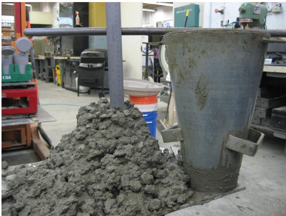
Figure 22(b) 0.55PC23 after HRWRA addition
