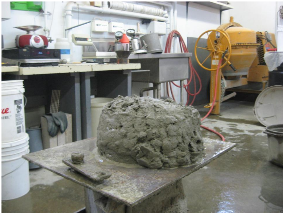
Figure 22(d) 0.55FA25 after HRWRA addition
