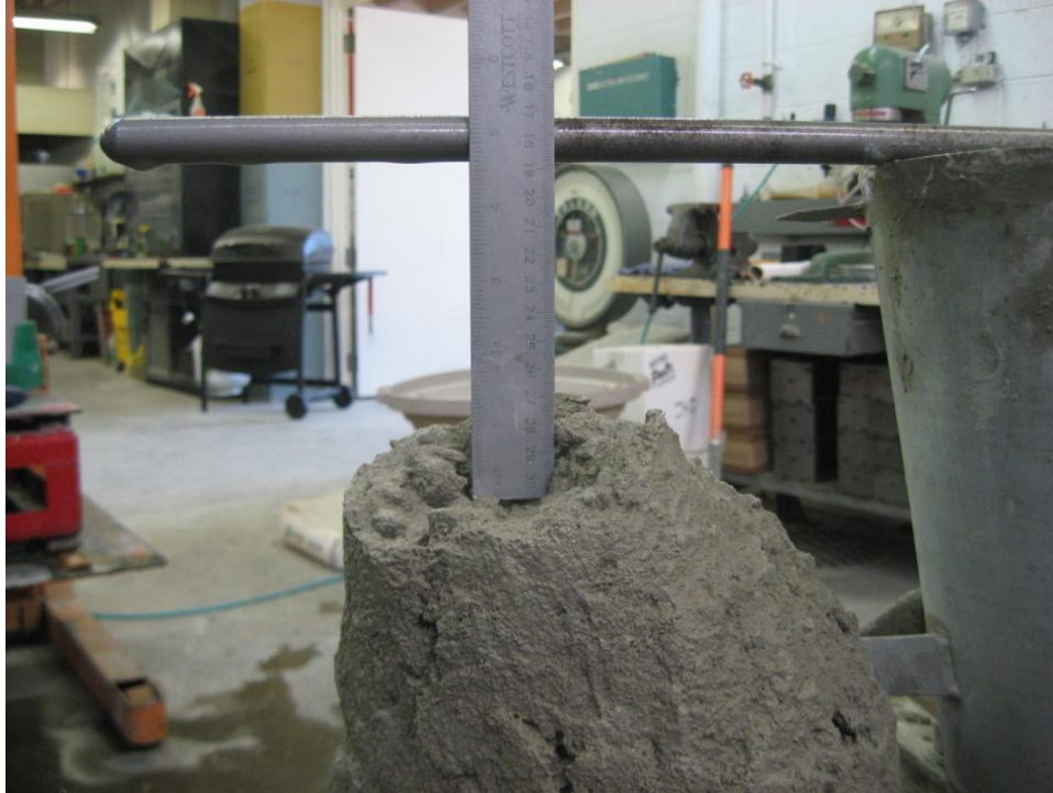
Figure 19(g) 0.47SL24A after HRWRA addition
