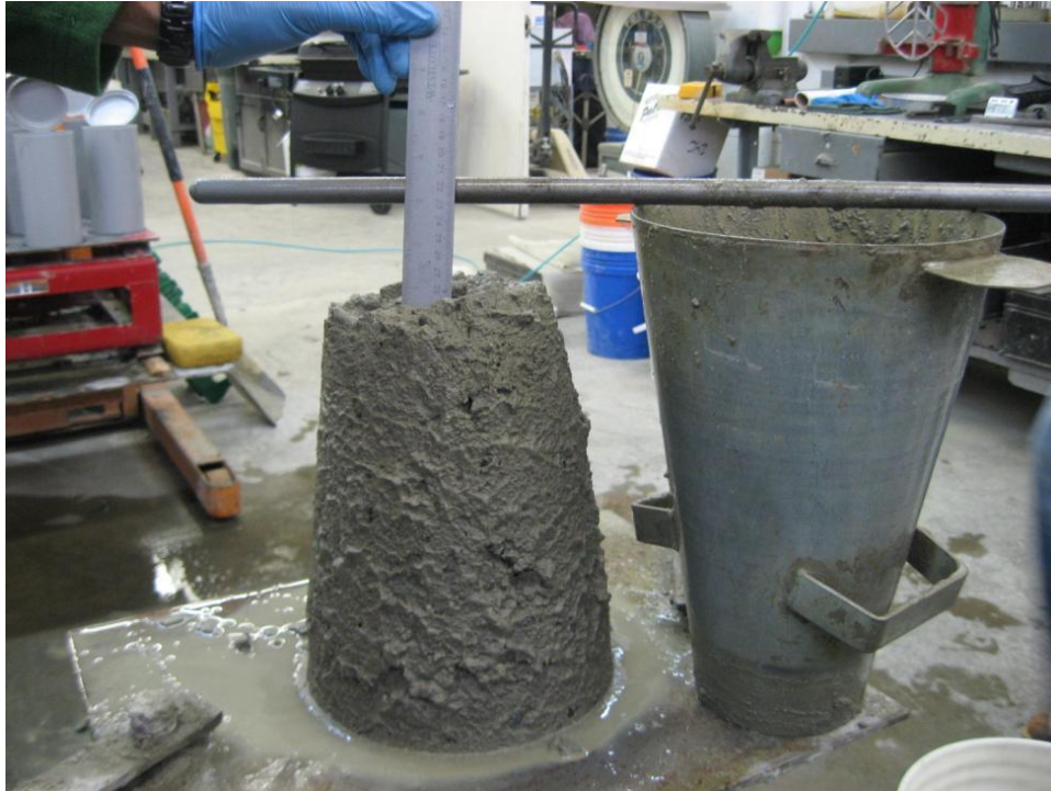
Figure 22(c) 0.55FA23 after HRWRA addition
