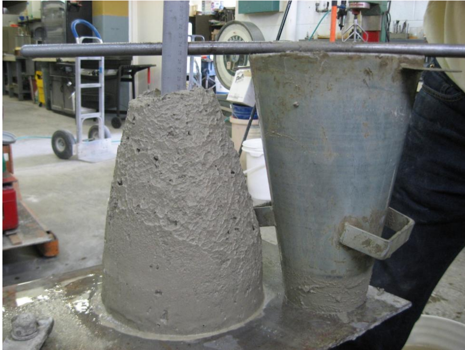
Figure 19(c) 0.47SL29A after HRWRA addition
