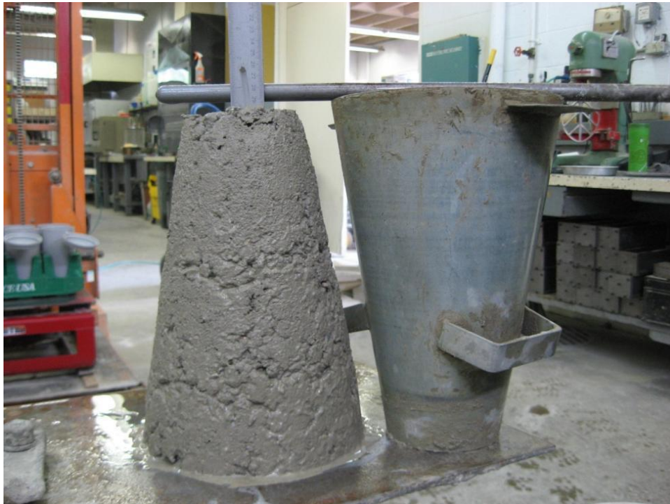
Figure 19(b) 0.47SL29A before HRWRA addition
