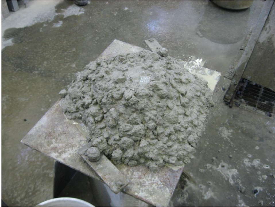
Figure 22(e) 0.40PC25 after HRWRA addition
