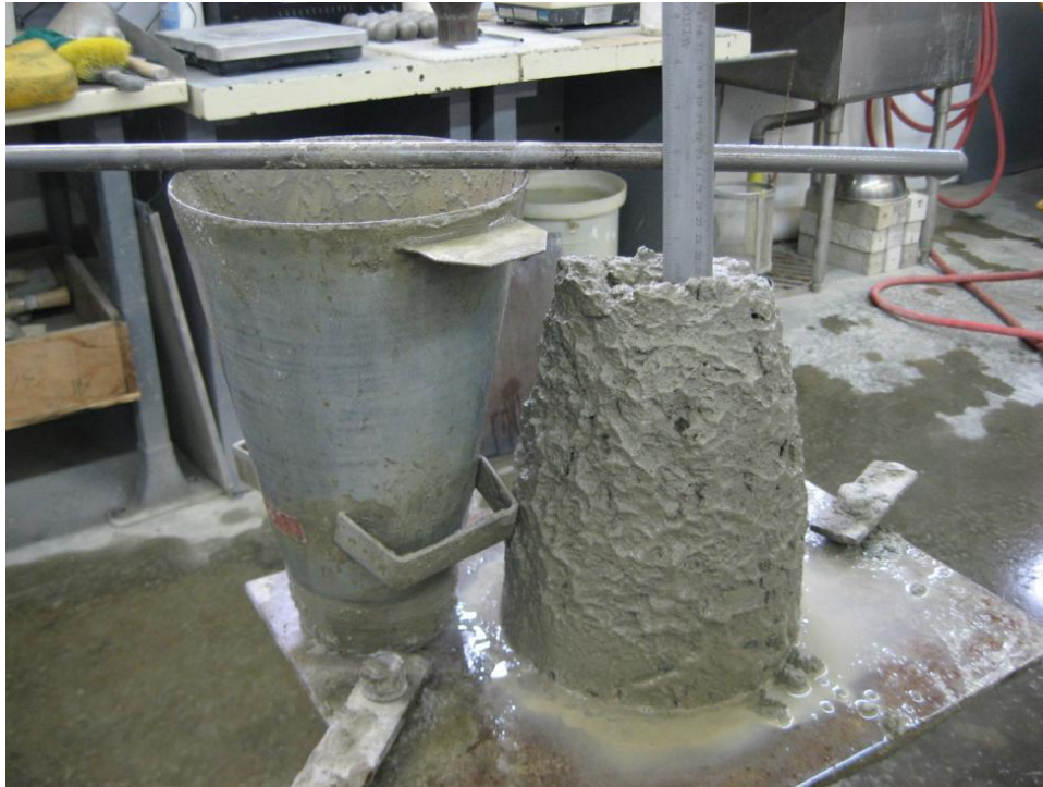
Figure 19(e) 0.47SL26A after HRWRA addition
