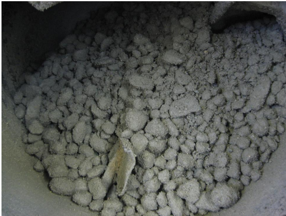
Figure 19(f) 0.47SL24A before HRWRA addition
