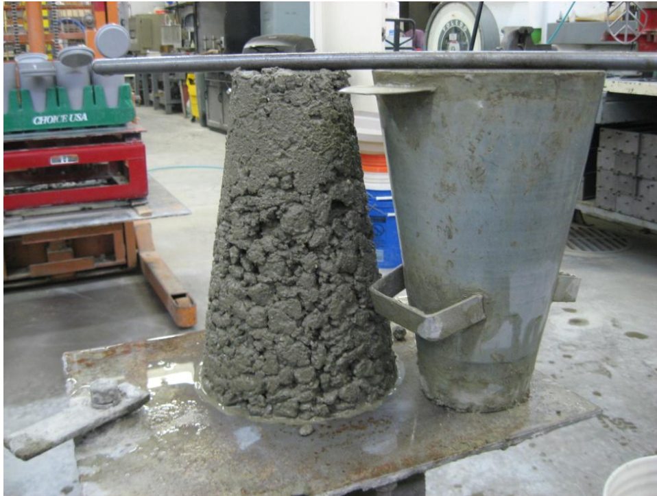
Figure 22(a) 0.55PC23 before HRWRA addition
