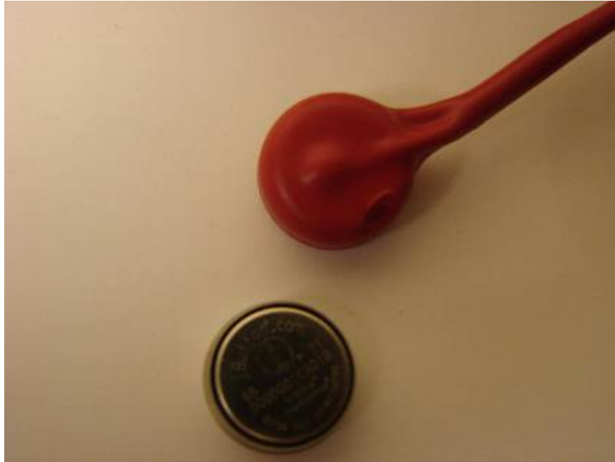
Figure 3.1 Temperature sensor (iButton®)
