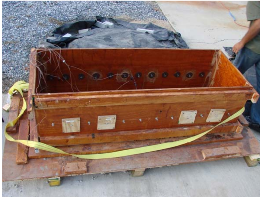
Figure 4.5 Field block with pullout inserts and temperature sensors
