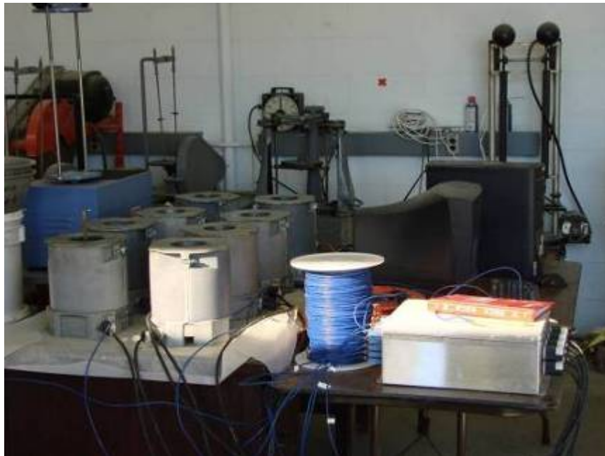
Figure 4.1 Match cure system showing 8 match-cured cylinder molds connected to a micro-controller computer
