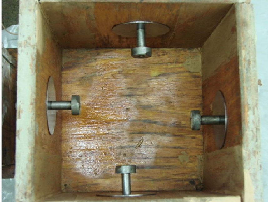
Figure 4.3 Cube molds with pullout inserts at the centers of the 4 side faces
