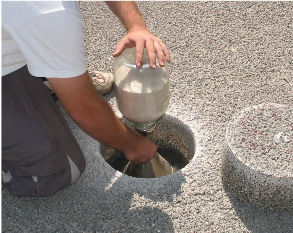
Figure 10: Performing Sand Cone Test
