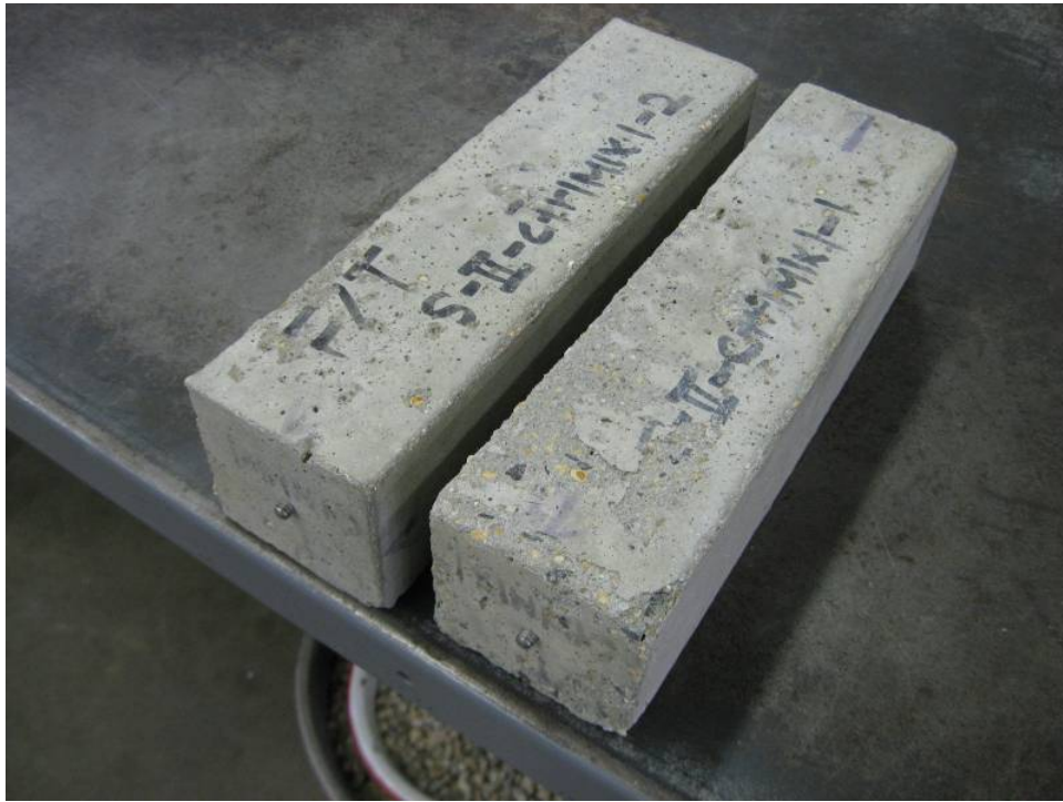
Figure 4. Control Mixture After 300 Freeze-thaw Cycles
