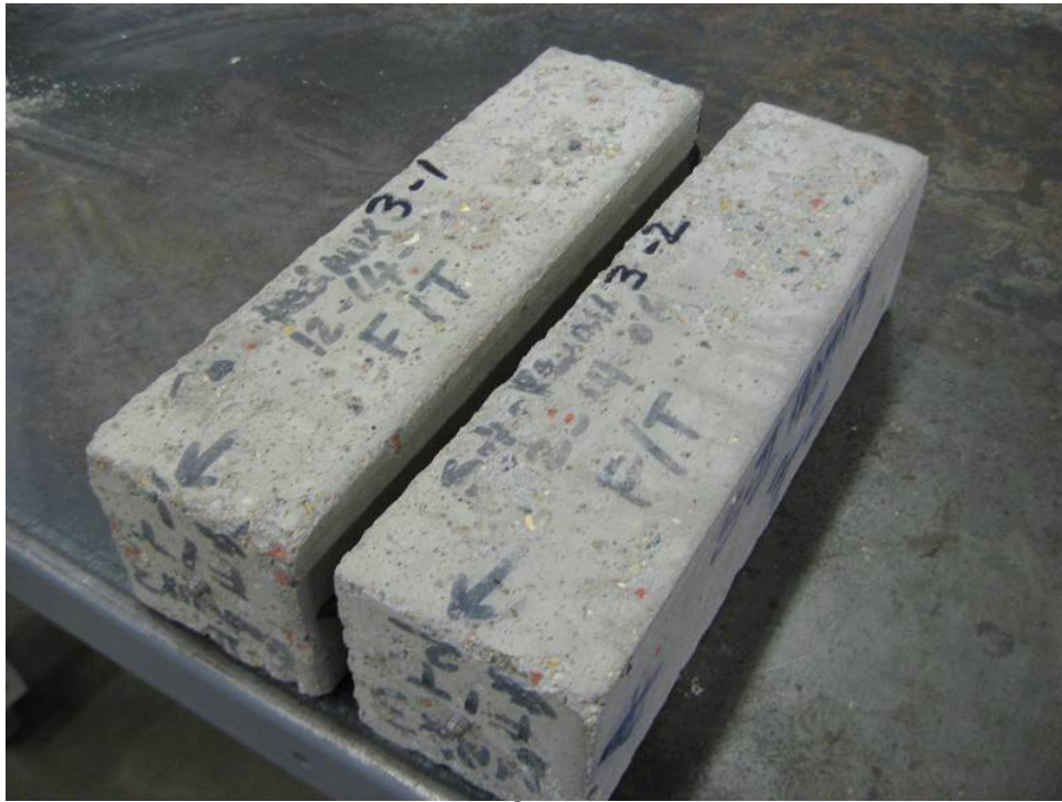
Figure 6. 3000 psi CCA at 600 lb/yd 3 Mixture After 300 Freeze-thaw Cycles
