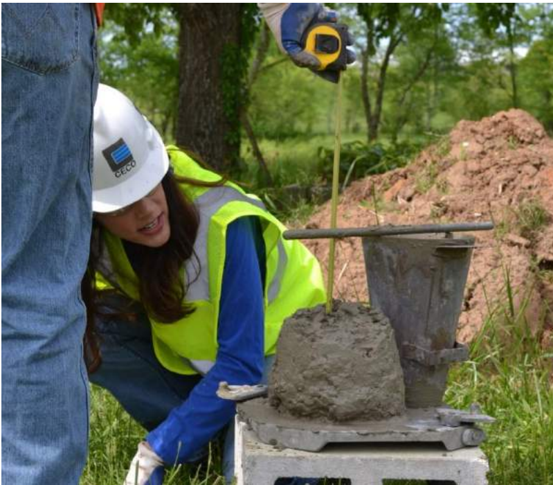
Photo 4. The 5½-in. slump proprietary wall mix had good cohesion
