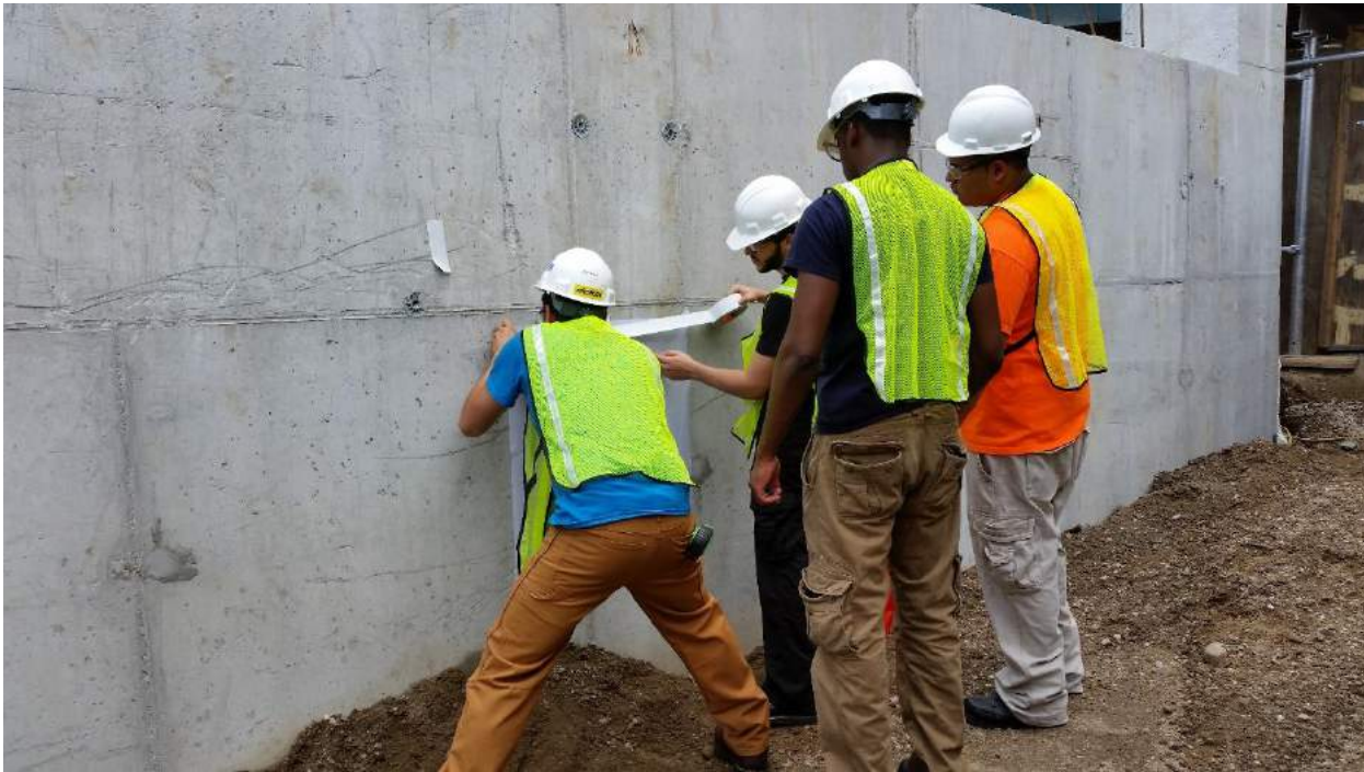
Photo 9. CIM student researchers mark off a randomly chosen 2x2-ft sample before measuring SVR for the sample surface.
