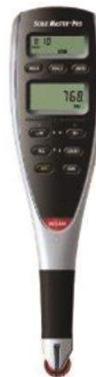
Digital measurement of bughole perimeter
