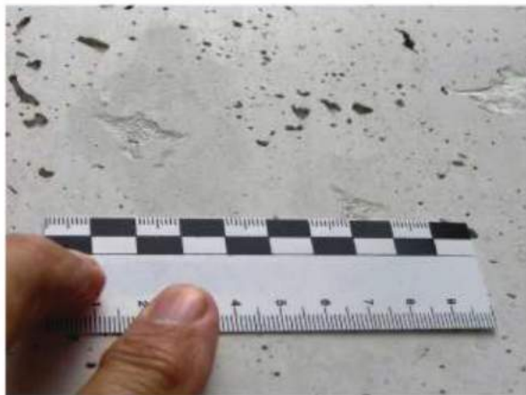
(b) Measurements of individual voids of (a)
