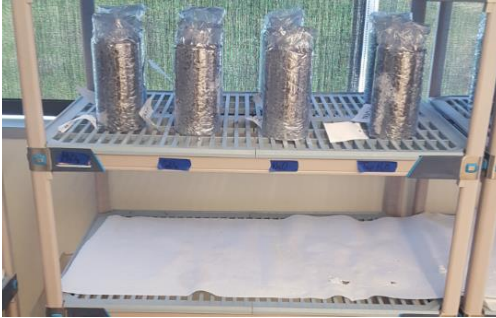
Figure 2.5: Photograph of a rack that held specimens in the ambient laboratory in between deicer applications with dripping pads below.
