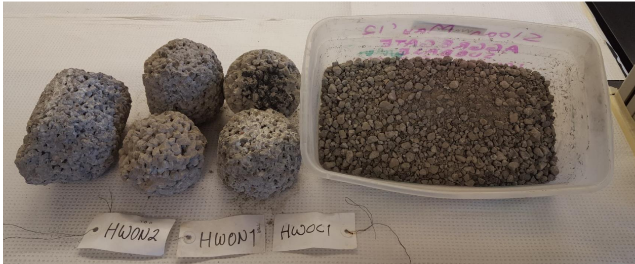
Figure 6.7: Abrasion test debris from three water specimens.
