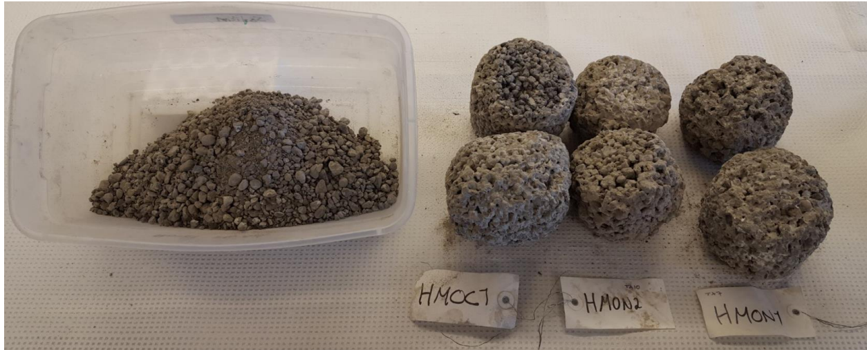
Figure 6.4: Abrasion test debris from three magnesium chloride specimens.
