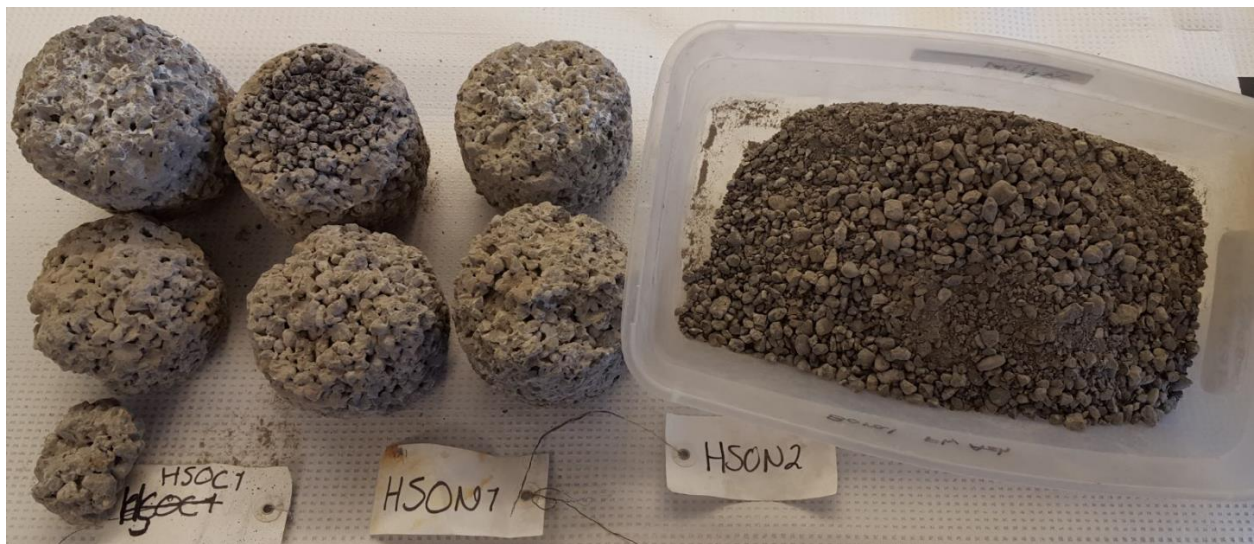
Figure 6.6: Abrasion test debris from three sodium chloride specimens.
