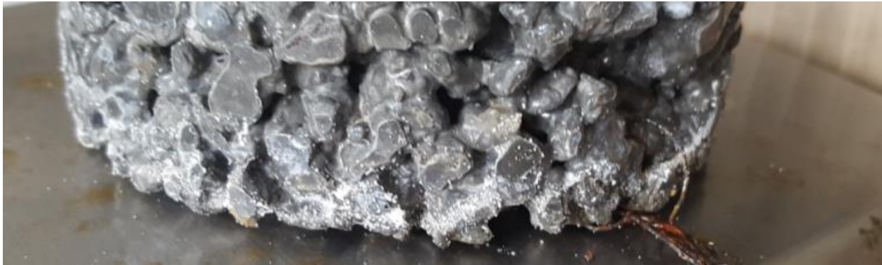
Figure 5.5: Solid precipitate formation on the bottom of a specimen subjected to magnesium chloride treatments.
