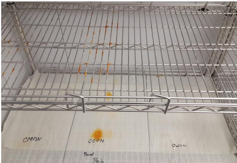
Figure 2.4: Photograph of a rack that held specimens in the cold room in between deicer applications with dripping pads below.
