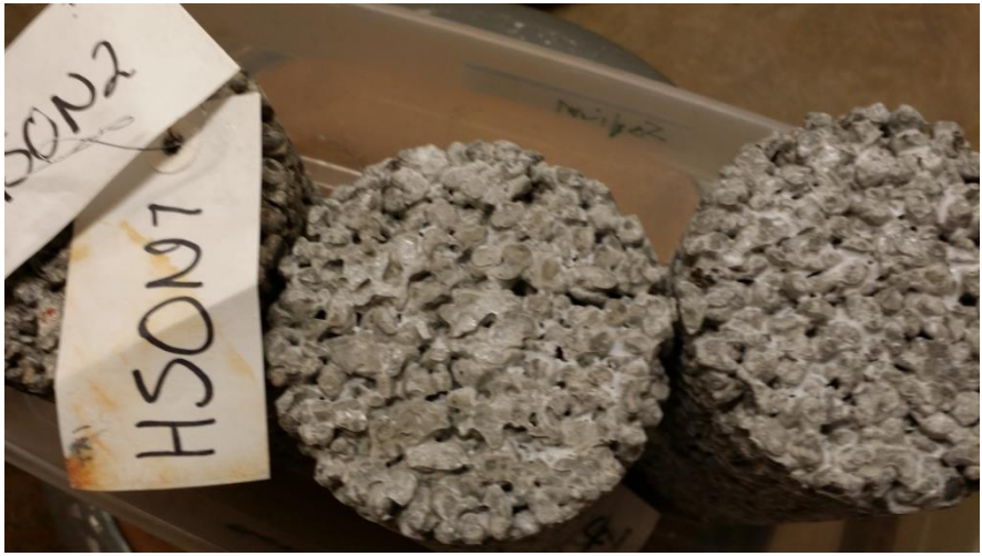
Figure 5.7: Solid precipitate formation on the bottom of three specimens subjected to sodium chloride treatments.
