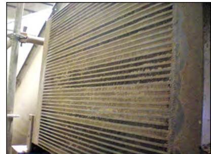
Photo 15-1: Dust can quickly clog radiators on windrow turners and other equipment, and lead to overheating © CH2M HILL
