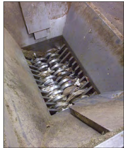
Photo 11-14: Cutting shafts inside a shear shredding unit © Scott Gamble
