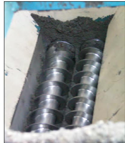
Photo 11-6: Top view of augers inside a horizontal mixer © CH2M HILL
