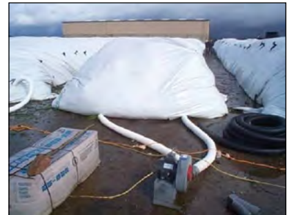
Photo 5-14: Composting system using polyethylene covers © Scott Gamble
