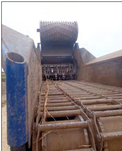
Photo 11-12: View of conveyor and grinding chamber of a horizontal grinder © CH2M HILL
