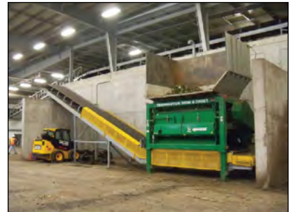
Photo 5-1: Shear shredders are commonly used to reduce particle size and further mix SSO feedstocks prior to composting © CH2M HILL
