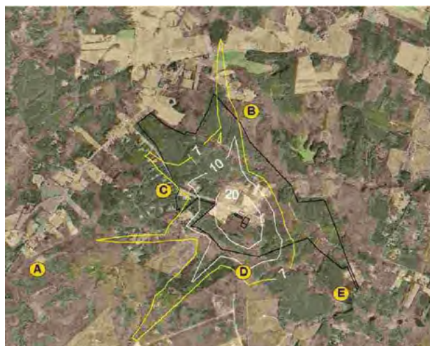
Figure 14-2: Odour model isopleths for planned composting operation © CH2M HILL
