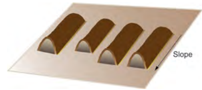
Figure 10-2: Windrow layout in a curing pad. Windrows should always be oriented in the same direction as the pad slope so drainage is not blocked.
