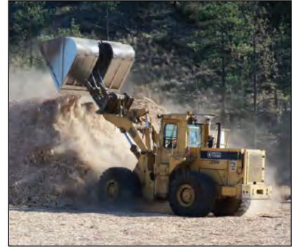
Photo 11-2: Front-end loader equipped with a roll-out bucket, which significantly enhances reach and versatility © CH2M HILL
