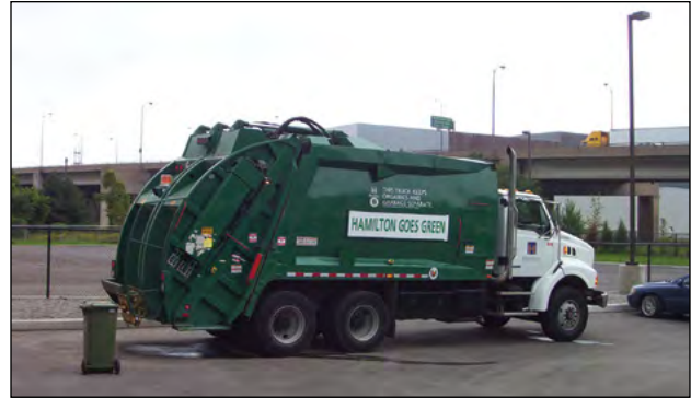
Photo 12-5: Dual-compartment truck that can be used to collect two different materials © CH2M HILL
