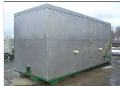
Photo 5-20: Static container composting system © CH2M HILL
