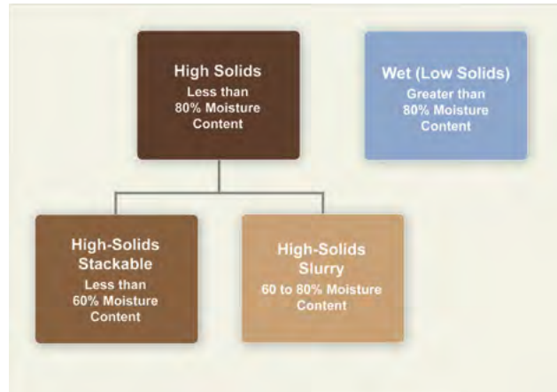
Figure 4-2: Types of SSO digesters
