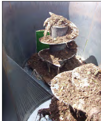
Photo 11-4: Augers inside a vertical mixer © Scott Gamble
