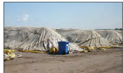
Photo 5-15: Covered, positively aerated composting system © CH2M HILL
