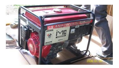
Generator used to pump the well - Honda 7600 IMC 240 (made in china)
