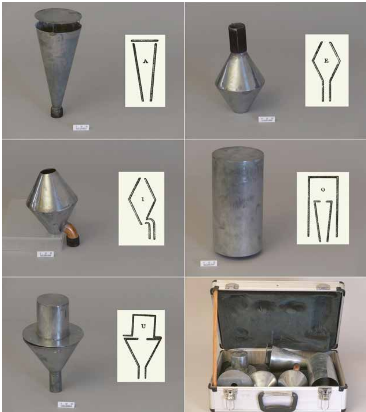
Figure 10. Korpiun's sheet zinc reproductions of Kratzenstein's five resonators, based on Thomas Young's illustrations from 1845. From Hoffmann (2021), pp.50–52. Courtesy of professor Rüdiger Hoffmann.
