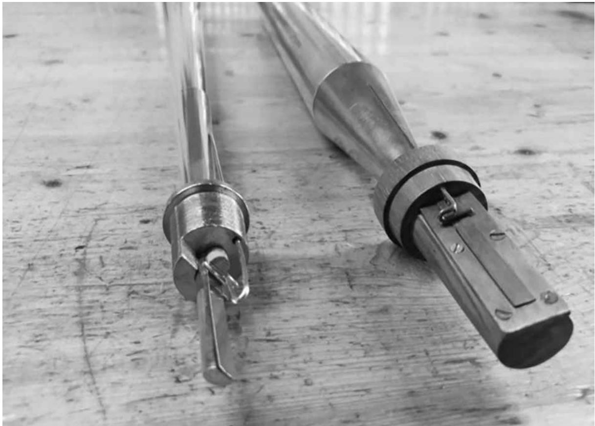
Figure 4. Organ voices with tuning springs, beating reed (left) and free reed (right). Made in 2022 by J.M. Fiskvik in Levanger, Norway for a new organ. Photo J.M. Fiskvik.
