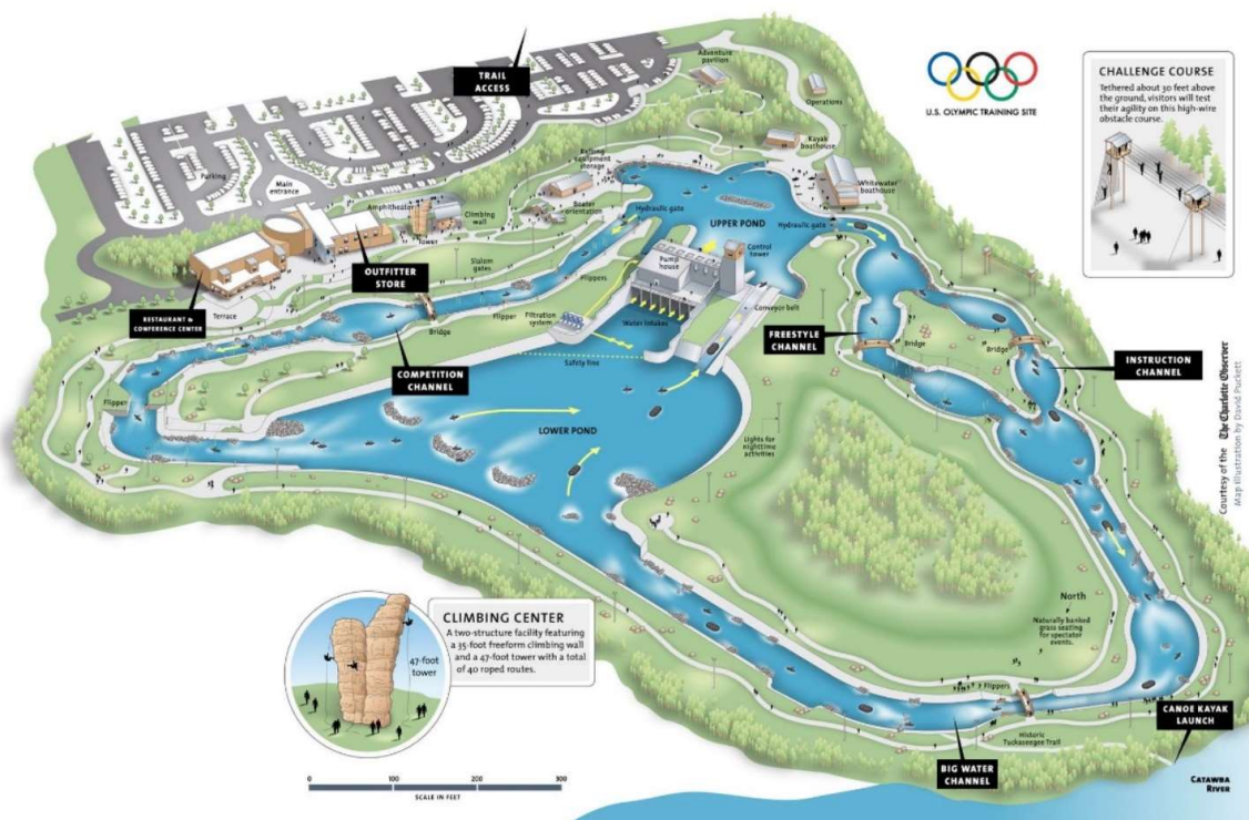
Figure 2: The US National Whitewater Center is a pumped whitewater park that pushes water from the bottom pond to the top where it then flows by the force of gravity through four channel segments.
