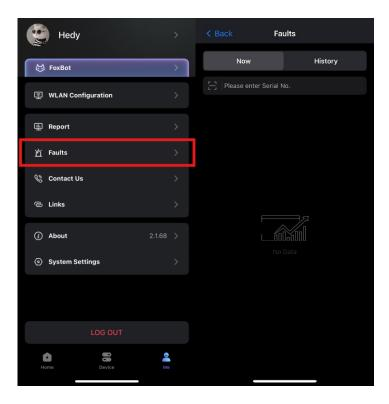
Note: For Option A, the Home page displays alarm messages related to that specific plant by default. For Option B, to view alarm messages in the Me page, you should first select the corresponding plant.
