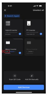
① The left number shows how many Micro Inverters are selected to connect to the network and the right number represents how many unconfigured Micro Inverters are detected.
