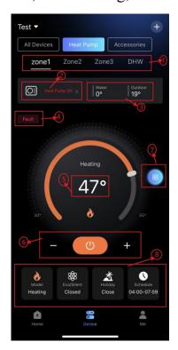
1 **Zone:** The heat pump system supports multi-zone control, allowing users to manage different areas of the building independently.
