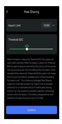
Peak Shaving requires setting two parameters: the Import Limit and Threshold SOC. When battery SOC is above the Threshold SOC, the system operates in Self-Use mode. Below this threshold, Peak Shaving activates: batteries discharge only when grid draw exceeds the Import Limit, while charging occurs from the grid during off-peak hours within
