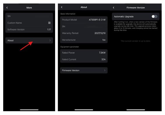
Note: After turning it on, new firmware versions will automatically upgrade during low-usage periods. The upgrade process requires 5-10 minutes, during which charging services remain unavailable.
