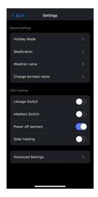
**Sterilization:** Perform a high-temperature cleaning cycle to eliminate harmful bacteria.
