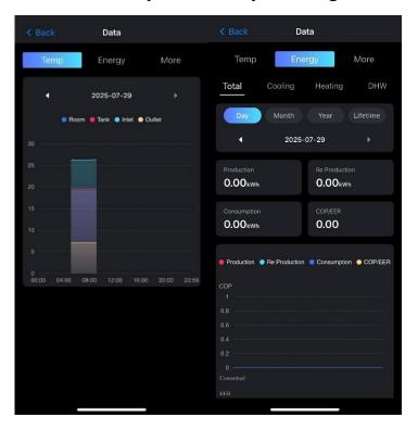
**COP** (Coefficient of Performance): Measure the heating efficiency of heat pump. It tells you how many units of heat energy are delivered for each unit of electrical energy consumed.
