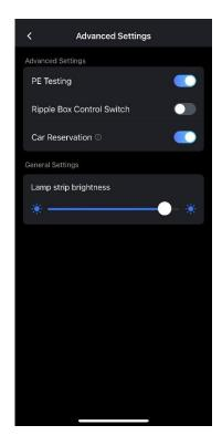
**PE Testing:** Check whether the protective earth connection is correctly installed and functioning.
