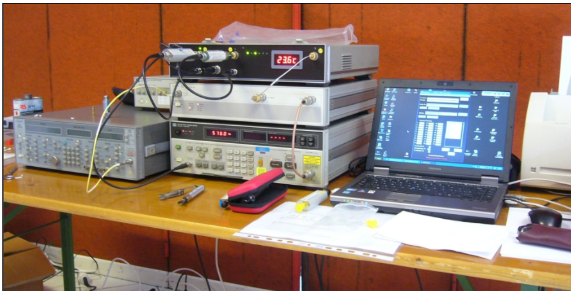
Fig. 6: Calibration in progress. Bottom to top: HP8970B, HP8971C and the home made unit with Reference and DUT noise sources.
