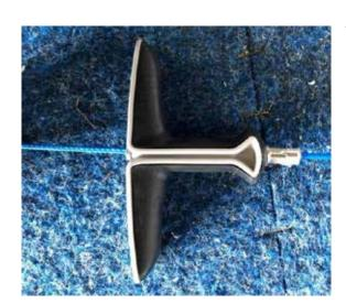
11. Fastern the bottom crimp using a crimping device.
