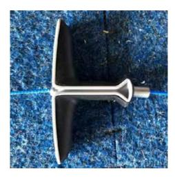
10. Slide the handle and bottom crimp such that the top crimp is flush inside the handle's recess and the bottom crimp is flush against the bottom of the handle
