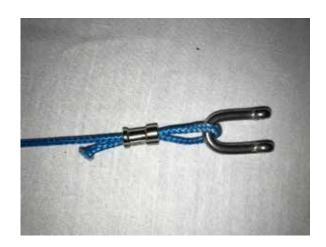
11. Slip the D-shackle through loop in synthetic cable/SS wire
