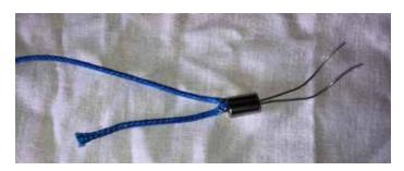
7. Slide the U-shaped piece of wire through the crimp so that the crimp is touching the bent section of the synthetic cable/SS wire
