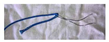
6. Loop end of synthetic cable/SS wire through the loop in the U-shaped piece of wire
