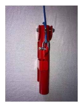
12. Fasten the D-shackle through the hole in the red handle. Damper flaps should be held fully open
