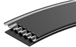
CMG with corrugated outer ring
