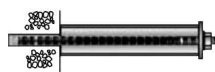
M16 threaded rod set in socket anchor and sheathed by tube under compression to avoid buckling
