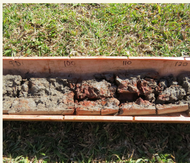
Image 2: Red mottles can be seen in this grey soil between 1 and 1.2 metres below the surface.
