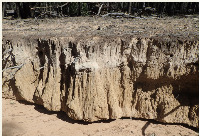
Image 3: Dispersive subsoils are very vulnerable to gully erosion.
