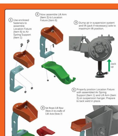
6 Rotate Beam Lift Base (Item 2) to proper position on air suspension beam and tack weld to lift arm (Item 3). Then, tack weld Beam Lift Base (Item 2) to suspension arm. Last, tack weld air spring support (Item 1) to hanger.
