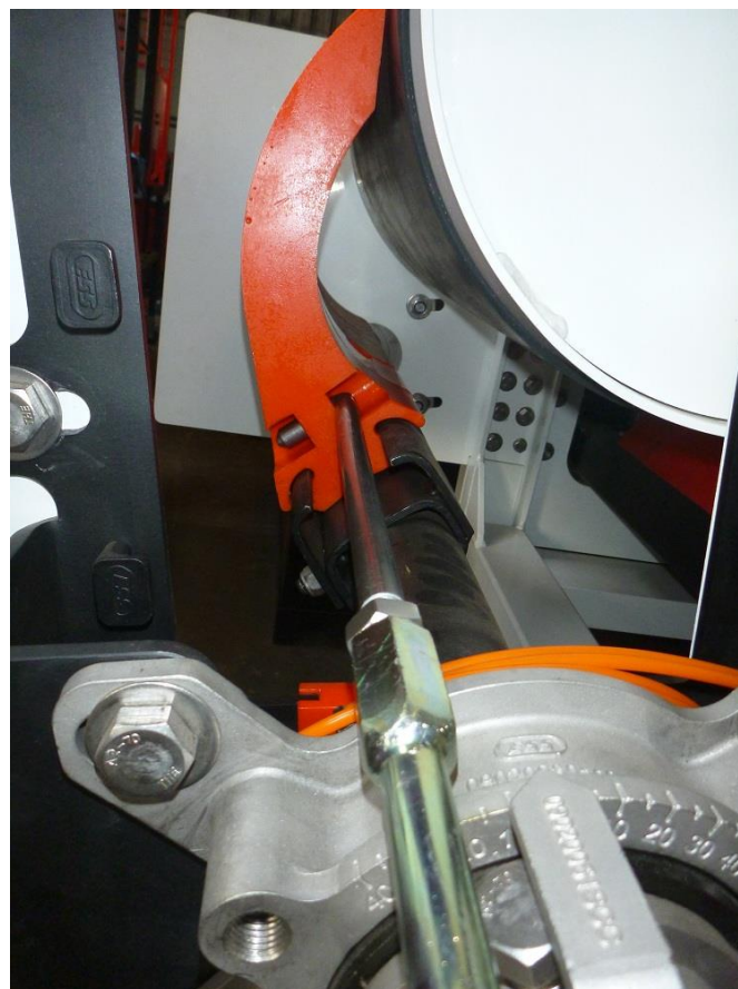
Figure 8– Keysafe 2 with Tool Tip Engaged and attached to Extraction Tool
