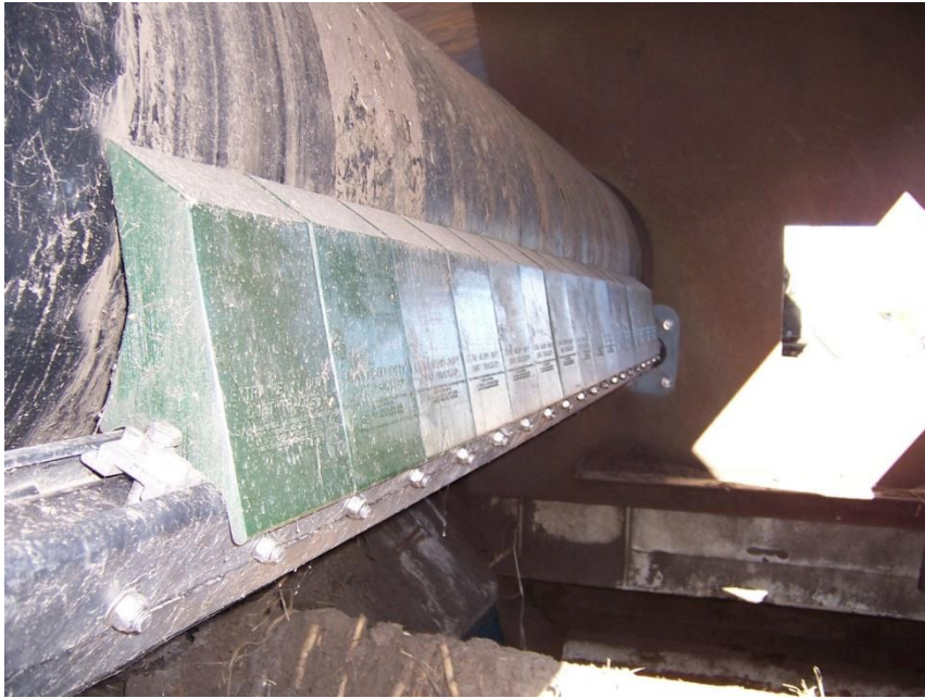
Figure 2 - XHD with Green Low Profile Blades on a Sugar Mill Bagasse Belt
