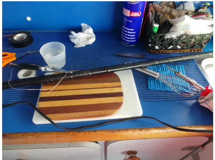
ABOVE: Making emergency repairs on board MV Trim . Note the use of the kitchen whisk to hold the hot soldering iron!
