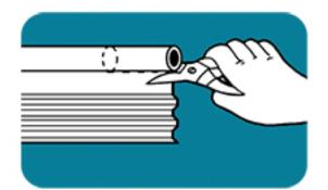
Cut off a 4 inch section of the round bead at the top of one of the edging pieces with a metal snip, utility knife or saw.
