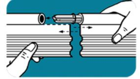
Use our exclusive crosslock connector to join the two sections, while overlapping the two pieces of edging.
