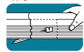
Drive 1 or 2 steel anchoring stakes through both sections at a 45 degree angle toward the turf or outside portion of the bed.
