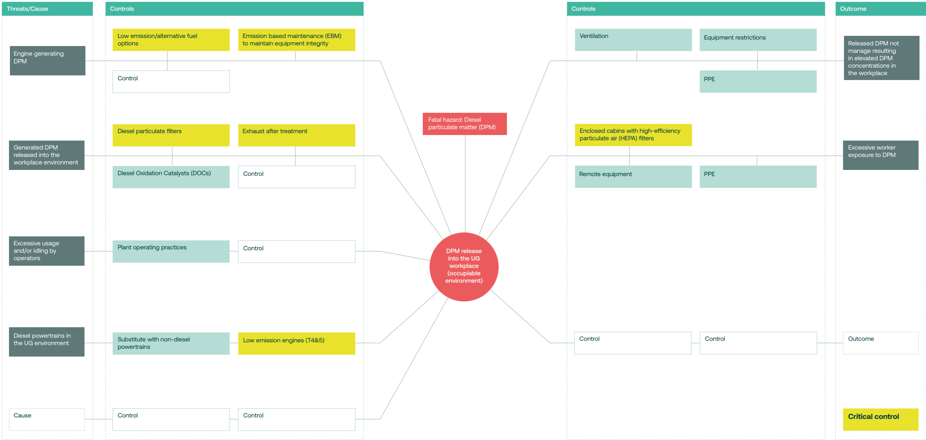
Figure 10: Example Bowtie – Diesel Particulate Matter Exposure
