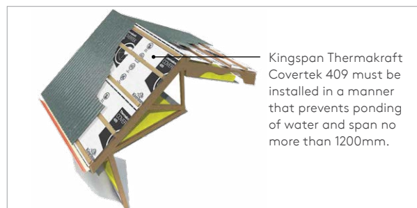
Figure 2. Kingspan Thermakraft Covertex 409 cavity fix method.
