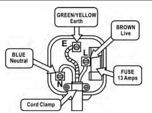
As the colours of the wires in the mains lead of this appliance may not correspond with the colour markings identifying the terminals in your plug, proceed as follows.
