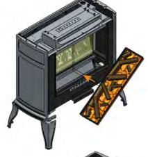
Ensure the glass is supported at all times! We strongly recommend protective gloves are used when handling glass.
