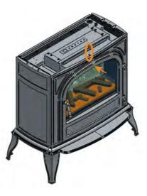
11) Screw the 4x M5 screws back into the position. Securing all the castings together.
