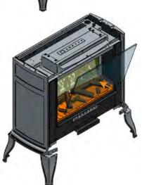
9) Screw the 4x firebox screws back into place, securing the glass and the retaining to the appliance.
