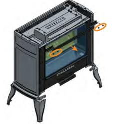
5) Carefully lift the glass up and out of the appliance and place safely on a soft, flat surface.
