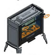
10) Screw the 1x M6 screw back into the top of the front casting.
