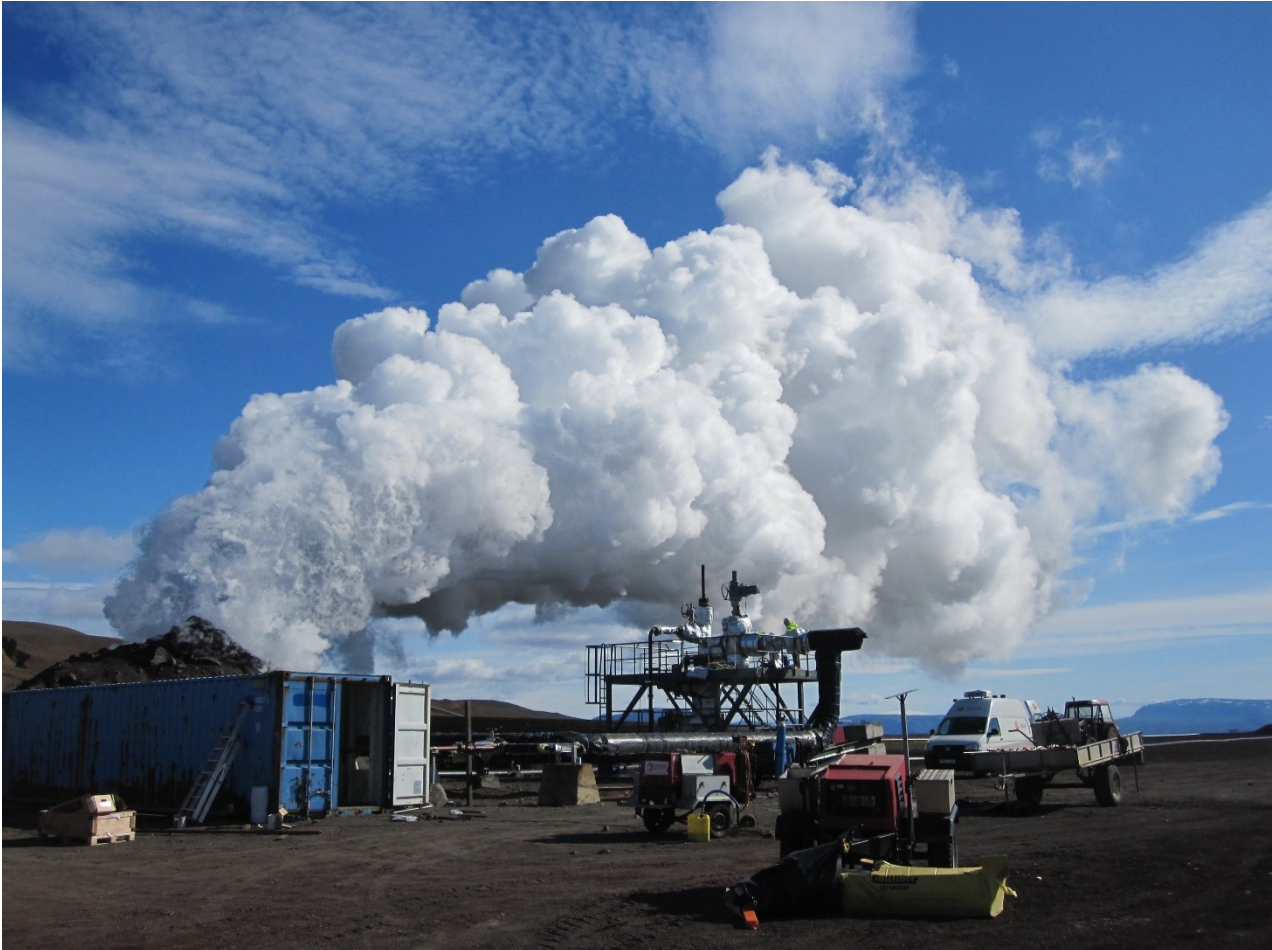
IDDP-1 being discharged in August 2012. Note the superheated steam at the top of the rock muffler (p. Kristján Einarsson).
