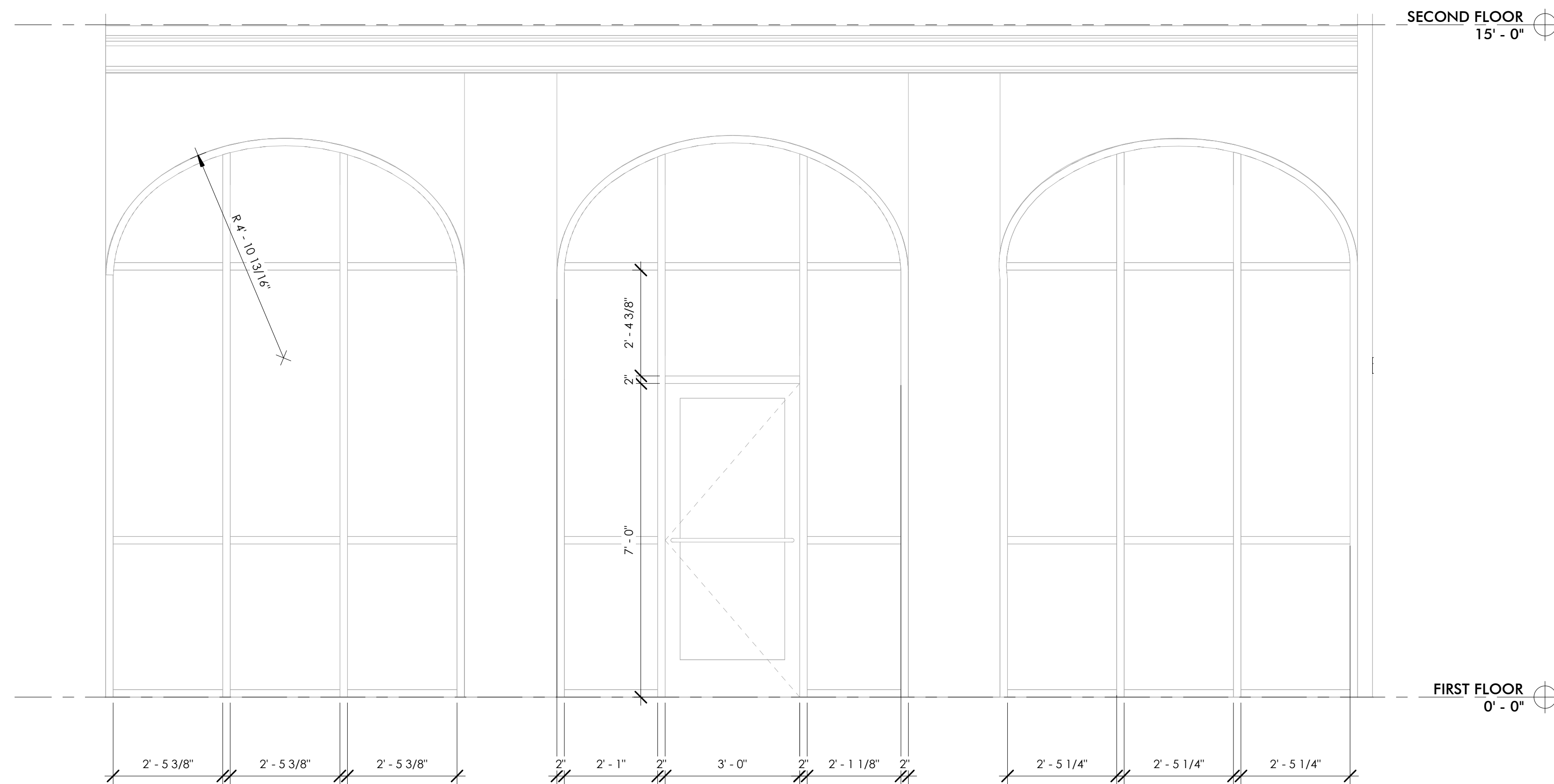
3 FRONT FACADE GLAZING DETAIL 1/2" = 1'-0"
