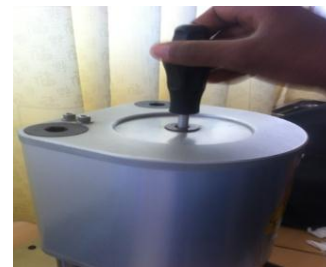
Figure 5. Packing of discharged material in the barrel
