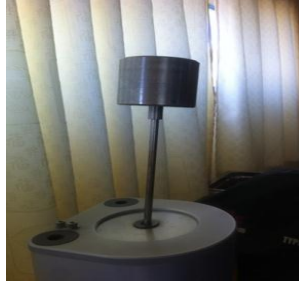
Figure 6. Position of dead weight in plastometer
