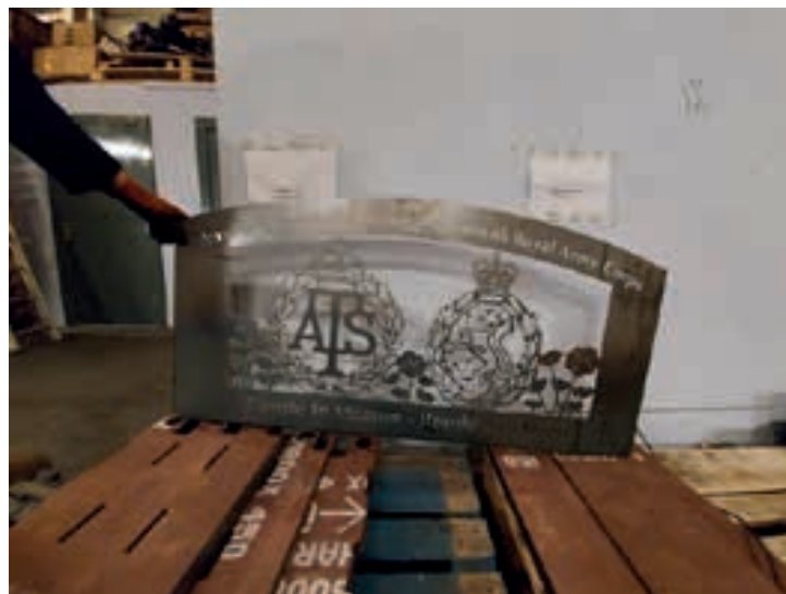
First stage of the bench. The steel solid steel sheet has been laser drawn. The next stage it is assembled into a complete steel bench. It will then be Powder coated
