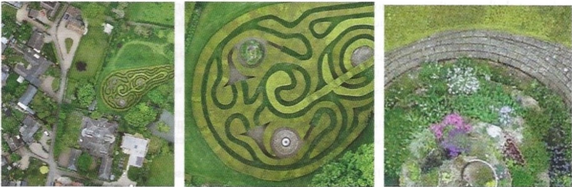
Figure 3. Image extracts from a survey flown in 2022 using a Wingtra drone processed to give a 3-cm pixel resolution (Copyright GeoInforma Ltd).
