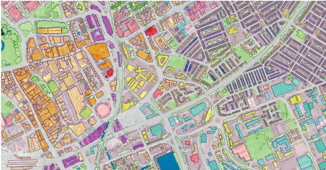
Above: Telcos will need a more detailed understanding of land and building use to engineer their 5G networks, using data such as this clutter map of Cardiff compiled for a Geomni UK customer
