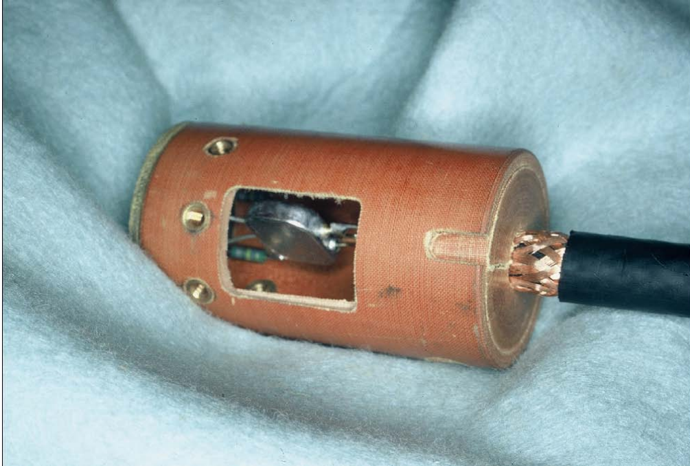
Figure 13. The 16-diode switch at top of each TeePee that rotates its excitation and changes its phase.
