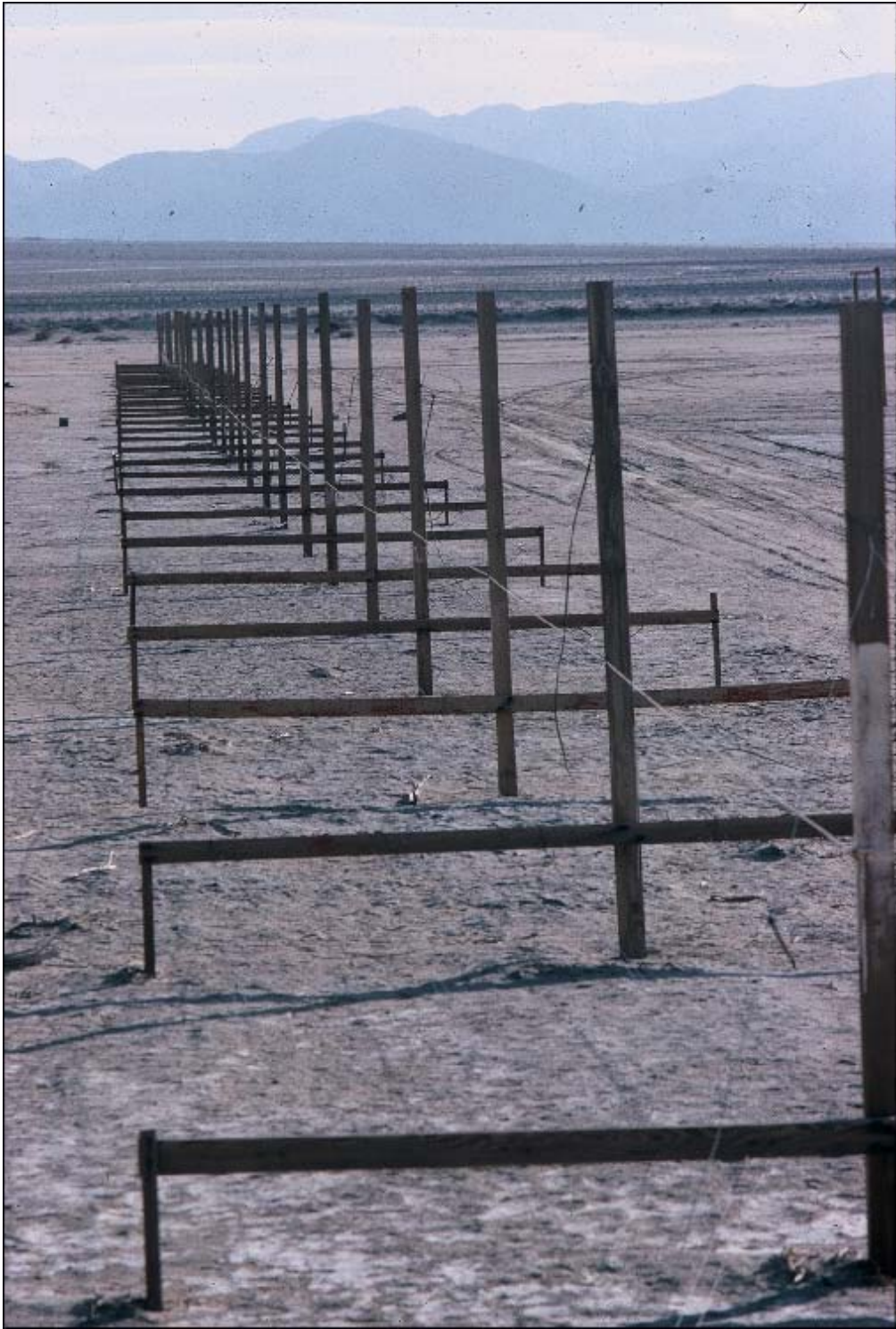
Figure 9. One of the grating arrays, each consisting of 19 colinear full-wave dipoles.
