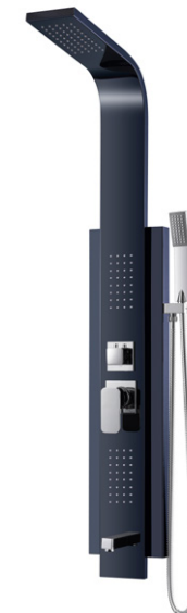
Y045B 1320*200*430mm 1.#304 stainless steel body in brush nickle finish 2.top shower 3.back massage nozzle 4.hand shower 5.Spout
