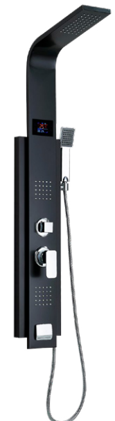
Y058 1295*250*425mm 1.#304 stainless steel body in black mirror finish 2.top shower 3.back massage nozzle 4.hand shower 5.spout
