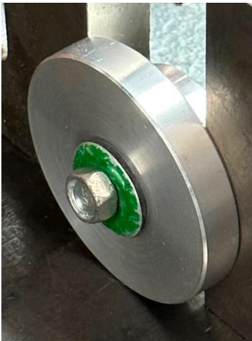
Release Bolt and Washer Correctly Tightened
