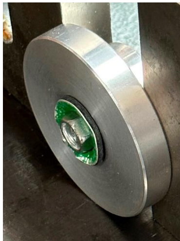
Release Bolt and Washer Over Tightened
