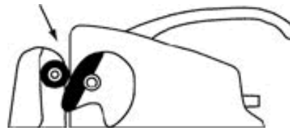
(#3) Cam in wrong position from improper strike mounting
