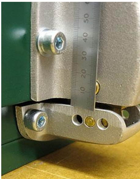
(#3) Cam in wrong position from improper strike mounting
