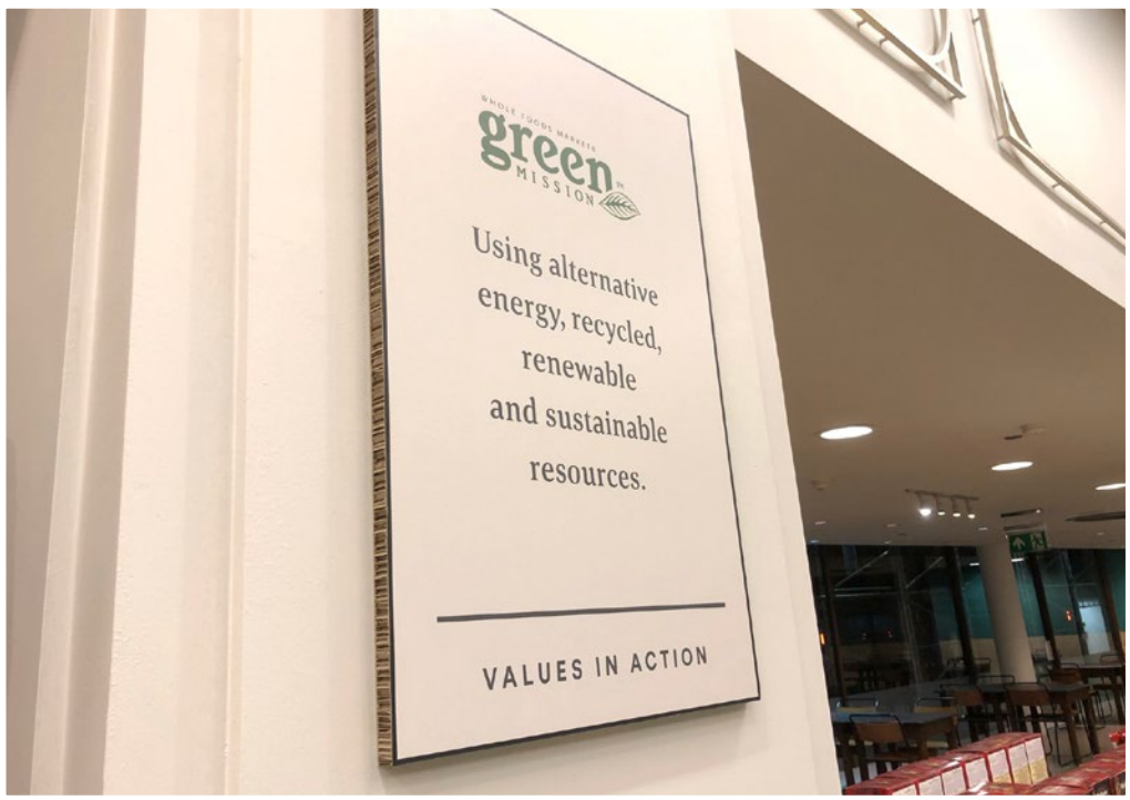
A Dufaylite panel, digitally direct to media printed in matt finish, installed using 3M RP45 VHB Tape
