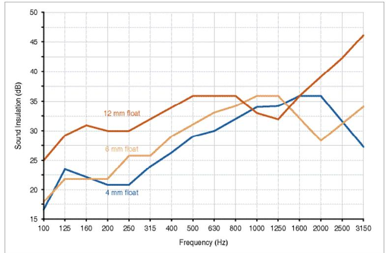
**Figure 3** Acoustic Performance of Float Glass
