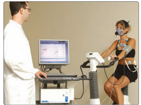
The CPET module add the possibility of performing pulmonary gas exchange analysis during exercise.
